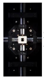
MuVi-SPIM system uses some unique and some patented technologies. The four objective lenses allow four combinations of illumination and detection. This provides four orthogonal views of the specimen without the need for sample rotation. It enables multiple view imaging of large samples at unprecedented speed with long-term stability.
